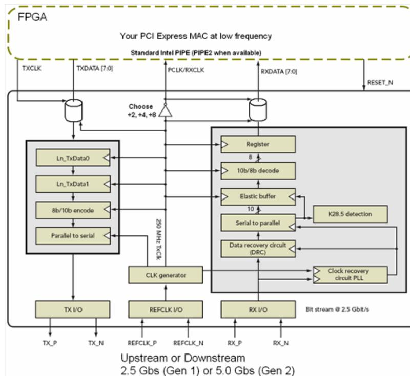
When connected between the user's design and the PCIe serial interface the Slowdown Core allows comfortable FPGA clock frequencies with 8 or 16-bit standard Intel PIPE interface. There is support for 1,4, and 8-lane configurations. No user MAC interface modifications are required, and developers now have a high speed method for complete design verification.
